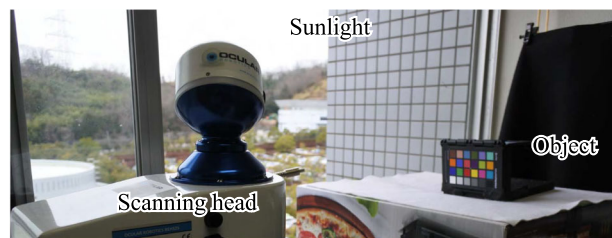
Fig. 3 Experimental setup. The scene is an uncontrollable environment near a window. Under a partly cloudy sky, the everchanging sunlight illuminates the color chart of the ColorChecker Passport
