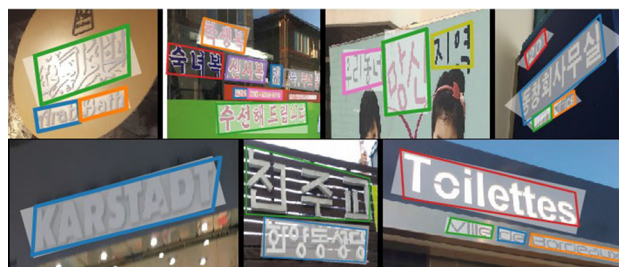
Fig. 8 Compared with the segmentation head, the proposed KE head predicts more compact bounding boxes and shows a higher recall rate for instances that were missed by segmentation. Colored quadrangles are the final detection results, whereas white transparent areas are the mask predictions grouped by the minimum area rectangle. (Color figure online)
