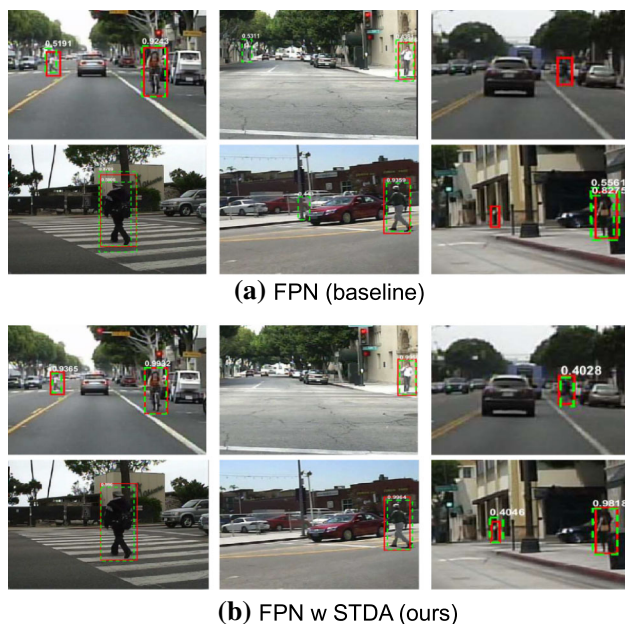
Fig. 11 Comparison of qualitative results about whether applying our method for dataset augmentation. Red boxes are ground-truths. Green dotted boxes are detection results. Best view in color
