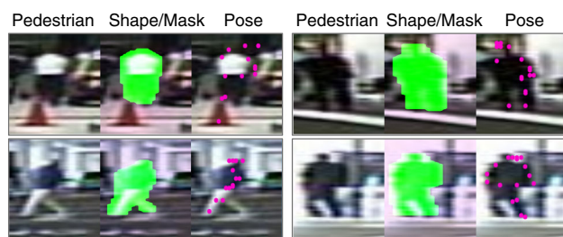
Fig. 2 Some examples showing that the shape estimation results are more accurate than pose estimation results on low-quality images using the same Mask RCNN model. Best view in color
