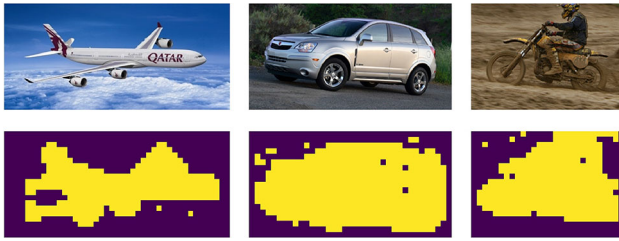
Fig. 6 Context segmentation results. A standard CompositionalNet learns a joint representation of the image including the context. Our context-aware CompositionalNet will separate the representation of the context from that of the object based on the illustrated segmentation masks
