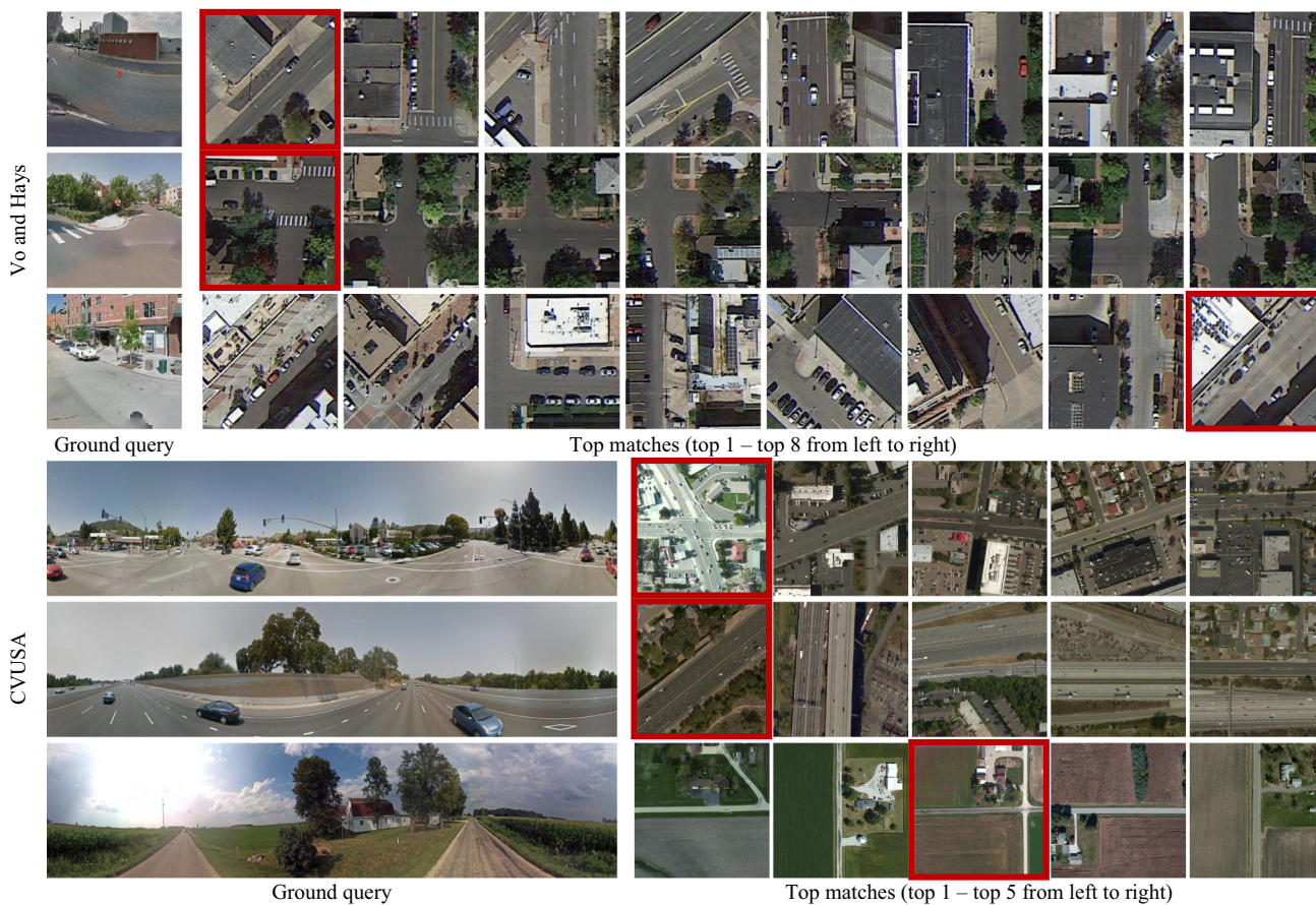
Fig. 8 Image retrieval examples on Vo and Hays dataset (Vo and Hays 2016) and CVUSA dataset (Zhai et al. 2017). The satellite image bordered by red square is the groundtruth
