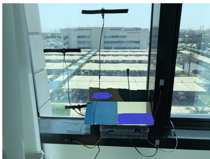
Fig. 9 Assembly of the Arduino boards and sensors in offices
