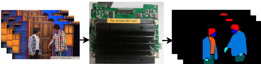
Fig. 1 Illustration of multi-human parsing using our method on Edge devices (Jetson Nano)
