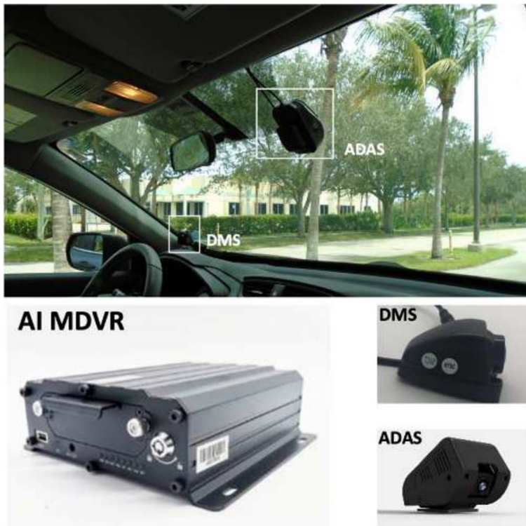
Fig. 3 In-Vehicle Vision Sensors, 2 Cameras + MDVR
