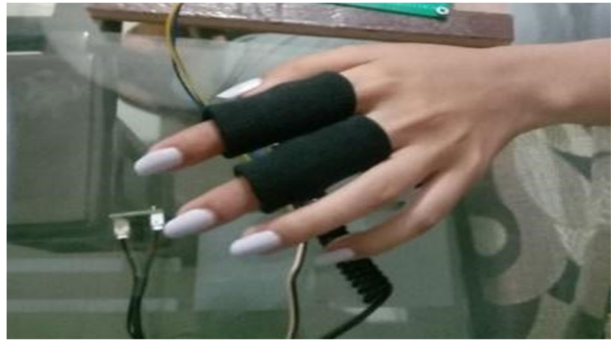
Fig. 6 Recording emotion data of subject using GSR sensor
