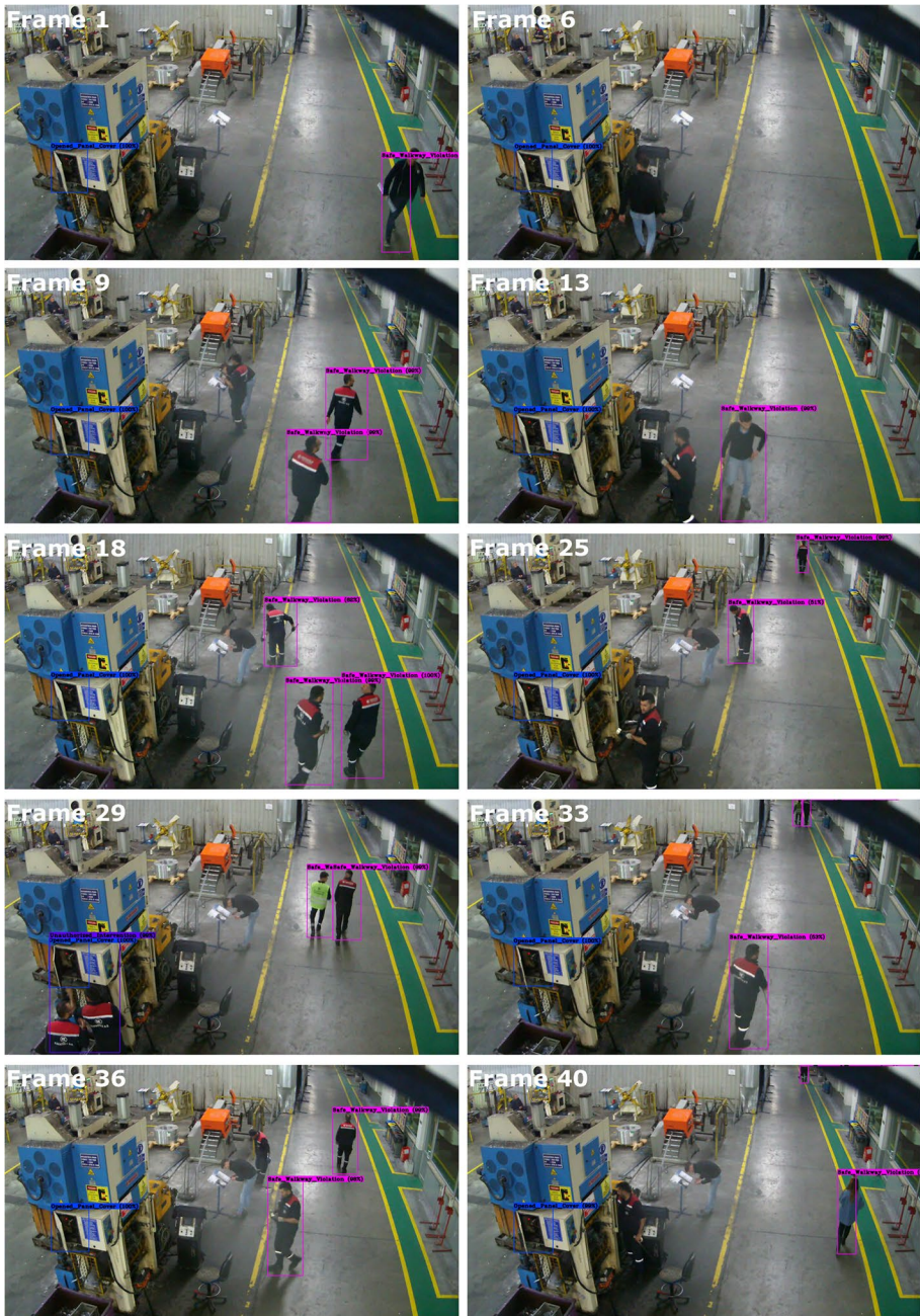
Fig. 10 A video fragment initially consisting of 105 frames, after passing through the YOLO v4 network, becomes a fragment consisting of 3 actions (unsafe behaviour) and 40 frames, and some sample frames in the reduced video
