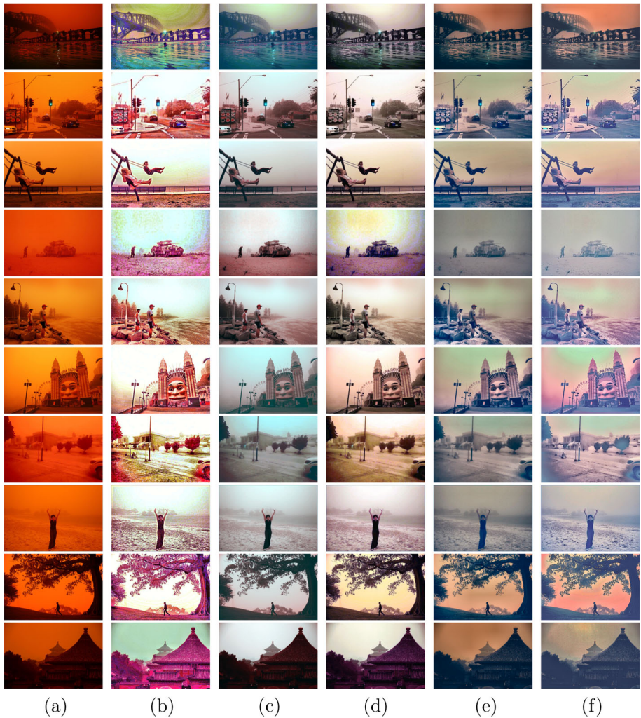
Fig. 6 Enhanced sand-dust images with extreme sand-dust color cast. (a) Sand-dust image, (b) Proposed method ( \alpha = 0.5 ), (c) Park and Eom [4], (d) Wang et al. [3], (e) Shi et al. [14], (f) Shi et al. [12]
