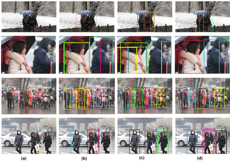
Fig. 10 Visualization results of dense pedestrians in bad weather. (a) stands for the original images, (b) stands for FPN detection results, (c) stands for CrowdDet baseline detection results, and (d) stands for our method detection results. The yellow dashed line indicates false positive instances, while the red dashed line indicates false negatives
