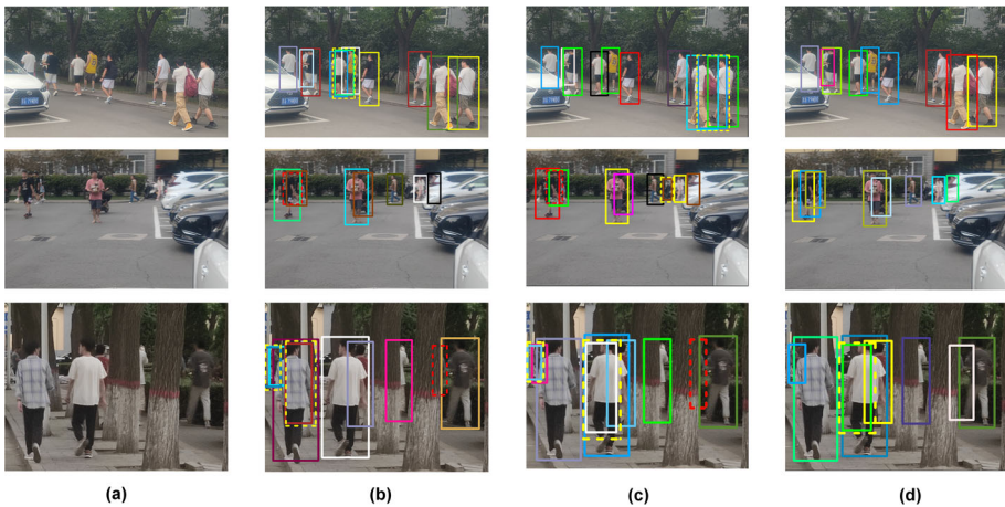
Fig. 9 Visualization results of dense pedestrians in realistic scenarios. (a) stands for the original images, (b) stands for FPN detection results, (c) stands for CrowdDet baseline detection results, and (d) stands for our method detection results. The yellow dashed line indicates false positive instances, while the red dashed line indicates false negatives
