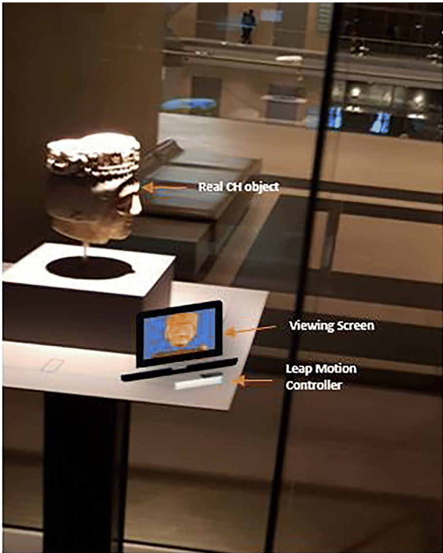
Fig. 5 A typical usage scenario of our system where a screen is stationed next to a protected cultural object. By means of a leap motion controller, and our 3D interaction software, a museum visitor can interact with the asset in a virtual environment using his bare hands
