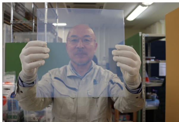
Fig. 5 Appearance of 300 \times 300 \times 8 \text{ mm}^3 aerogel monolith obtained by ambient pressure drying
