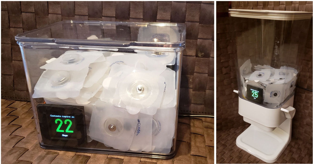
Fig. 1 Devices for Storage, Dispensing, and Shelf-Life Tracking of Electrocardiography Electrodes
