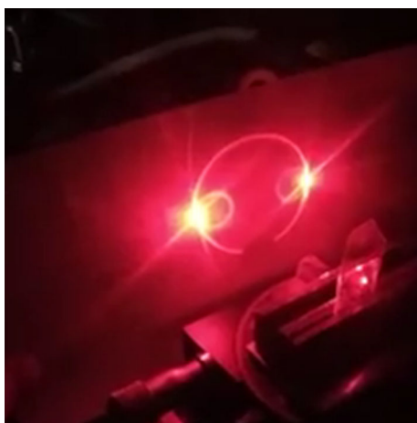
Figure 10 A photo of the diffraction pattern of a hologram recorded in a photopolymer with a DT monomer.
