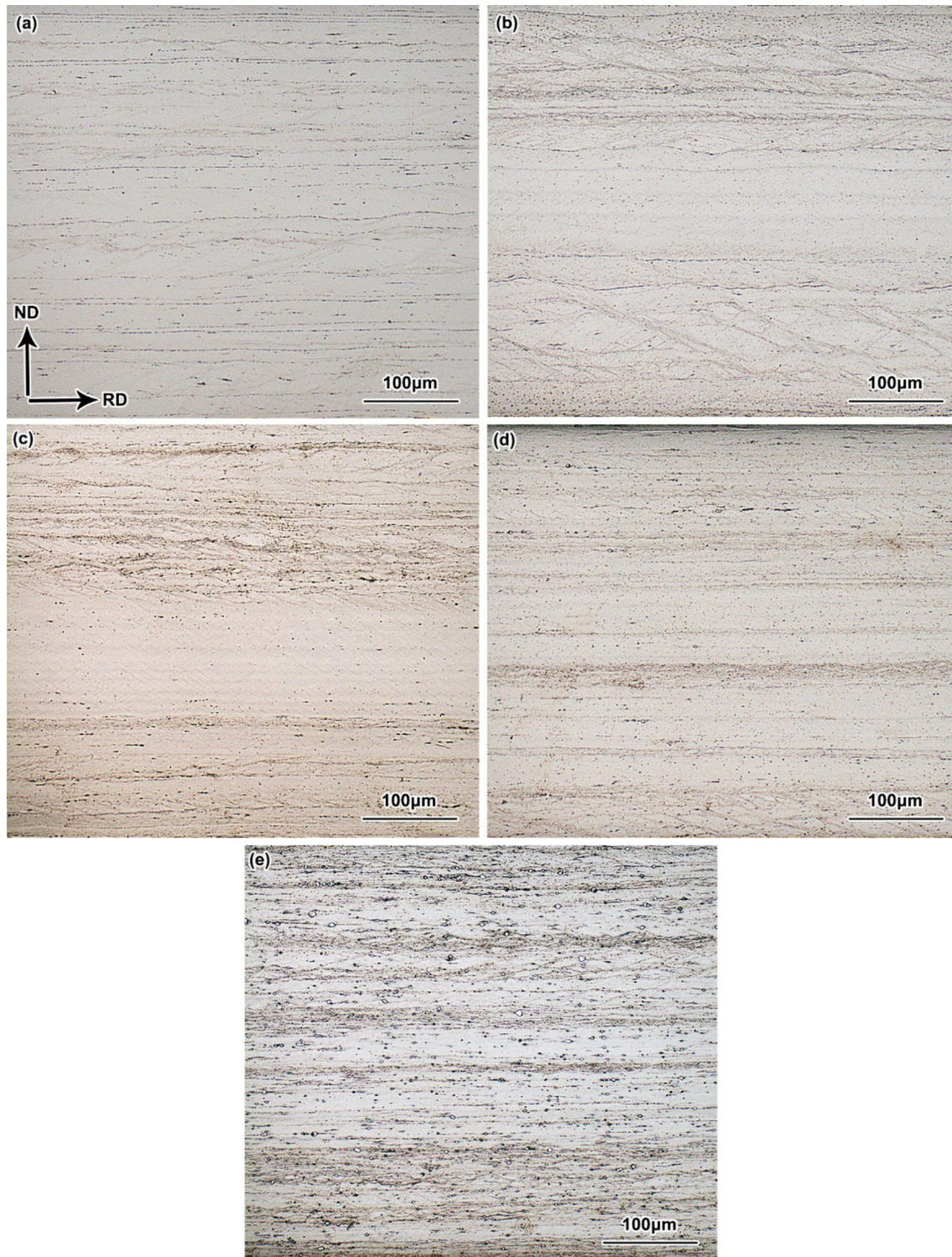
Figure 3 Microstructure of warm-rolled sheets of high-silicon electrical steel with different Nb contents: a 0wt%Nb; b 0.05wt%Nb; c 0.10wt%Nb; d 0.15wt%Nb; e 0.50wt%Nb.
