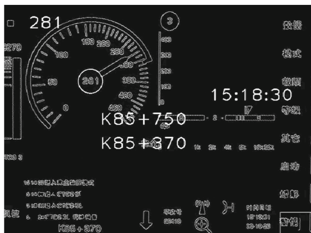
Fig. 2 DMI image with tilt correction and recognition
