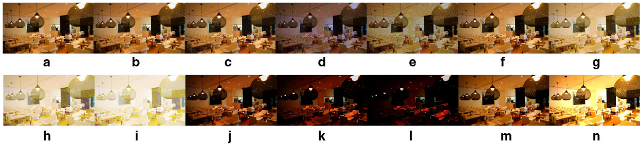
Fig. 1 Example of the image distortions applied in the evaluation of the robustness of CNN-based image recognition models: a Original image, b JPEG over-compression, c Additive White Gaussian Noise,
