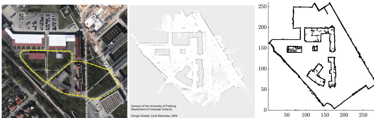
Fig. 11 The left picture shows the satellite map of the Freiburg University Campus where the yellow dashed line indicate the robot trajectory. The middle figure shows the corresponding occupancy map of the
