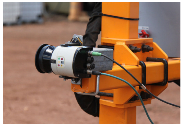
(b) 2D SICK laser vertically-mounted.
