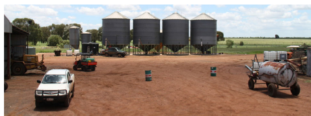
Fig. 14 Set up for hardware experiment 1 with 5 objects (ute, small utility vehicle, petrol tank on trailer, two drums). Robot start location is bottom-left corner and goal region is top-right corner. Size is 24 m × 36 m
