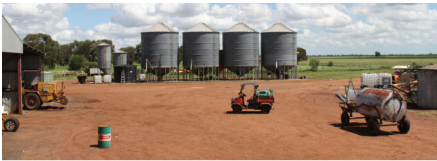
Fig. 17 Set up for hardware experiment 2 with 4 objects (small utility vehicle, petrol tank on trailer, two drums). Robot start location is bottom-left corner and goal region is top-left corner. Size is 24 m × 36 m
