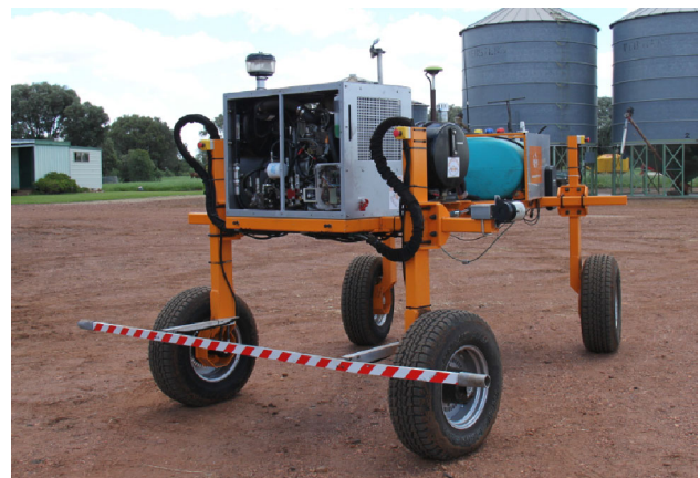
(a) Outdoor robot with LHD kinematics.
