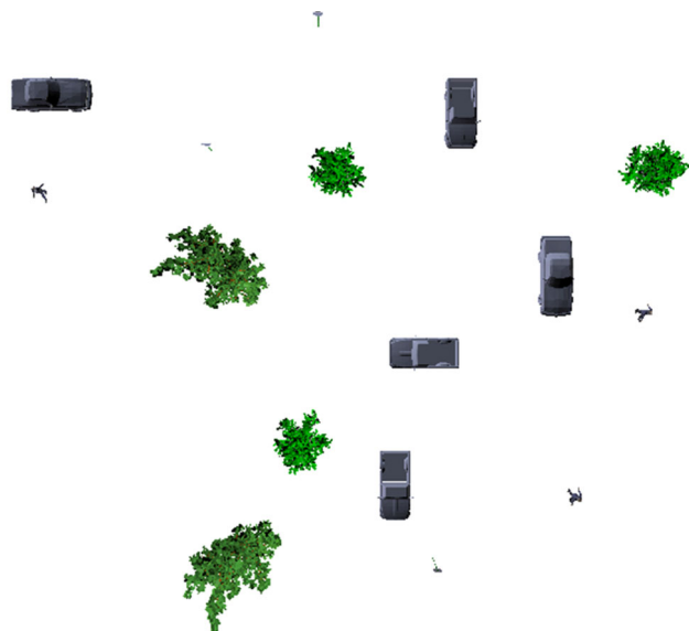
Fig. 8 Simulation environment 2 (corridor) with 16 objects. Robot start location is near bottom-left corner and goal location is near top-right corner. Size is 44 m × 44 m
