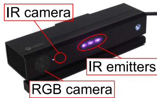
Fig. 12 The Kinect V2 sensor with IR camera, RGB camera and IR emitters
