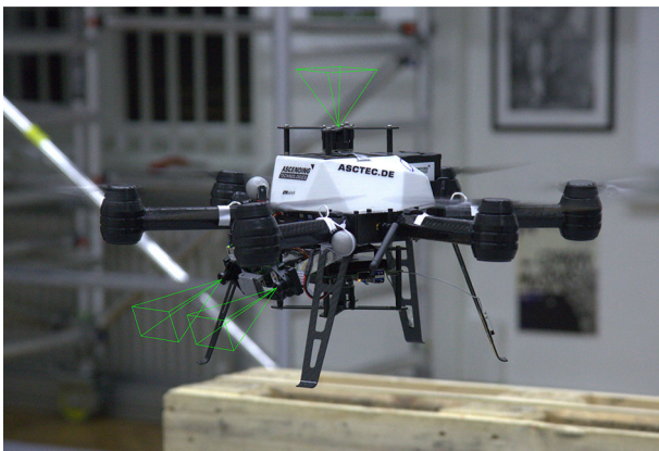
Fig. 11 The AscTec Neo hexacopter MAV is depicted, with the fields of view of the stereo camera pair and the upward facing camera visualized in green (Color figure online)
