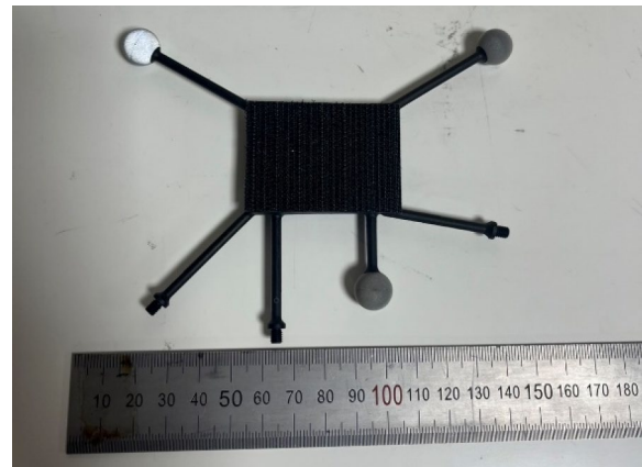
Fig. 4 Photograph of the marker with retro-reflective materials for tracking user movements
