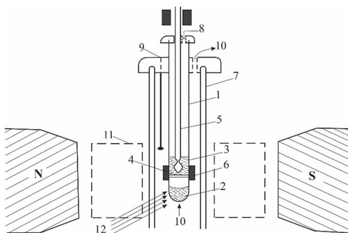
**Fig. 1** Experimental setup: (1) quartz cell; (2) solution of *tert*-butylOOH; (3) solution of antioxidant, chelate or phenolic compound; (4) tefflon membrane; (5) quartz stirring rod; (6) tefflon joint; (7) dewar; (8) dry air inlet; (9) thermocouple; (10) thermostating gas; (11) EPR cavity; and (12) UV irradiation photolysis source, [22, 23]
