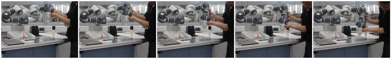
Fig. 8 Human demonstrations of rivet picking. During the human demonstrations, the YuMi robot is in lead-through model and the trajectories are captured using socket communication to an external PC
