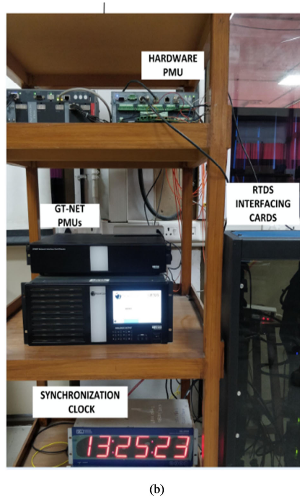
Fig. 6 a WSCC 9-Bus system model in RSCAD b RTDS-based experimental WAMS testbed c Communication between PMU and PDC using IEEE Standard C37.118 protocol in network monitoring tool Wireshark
