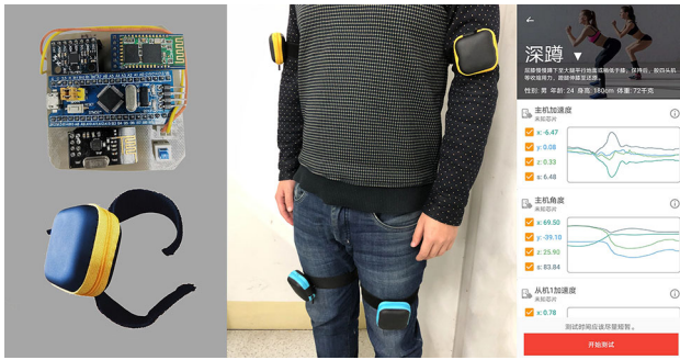
Fig. 3 The wearable microsensors; a participant wearing the devices; the app interface and data visualization
