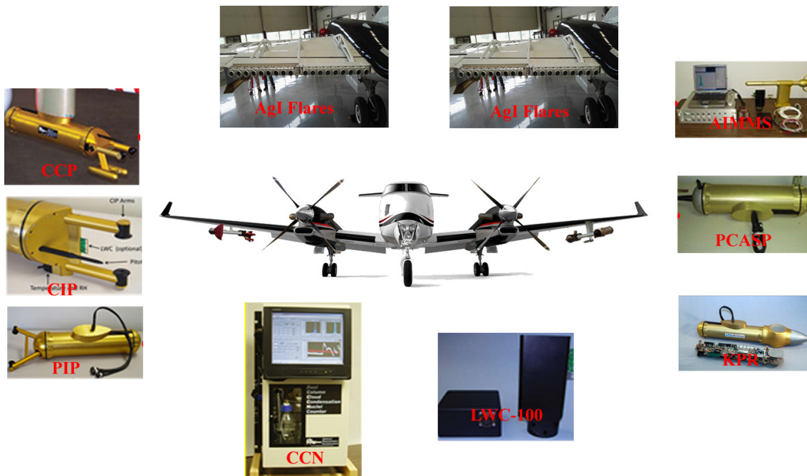
Fig. 1. Photos of the King Air aircraft probes, including AgI flares equipment, Ka-band cloud radar (KPR), cloud combination probe (CCP), cloud imaging probe (CIP), precipitation image probe (PIP), 20 Hz Aircraft-Integrated Meteorological Measurement System (AIMMS-20), Passive Cavity Aerosol Spectrometer Probe (PCASP), cloud condensation nuclei (CCN) counter and Hot-Wire Liquid Water Content Sensor (LWC-100).
