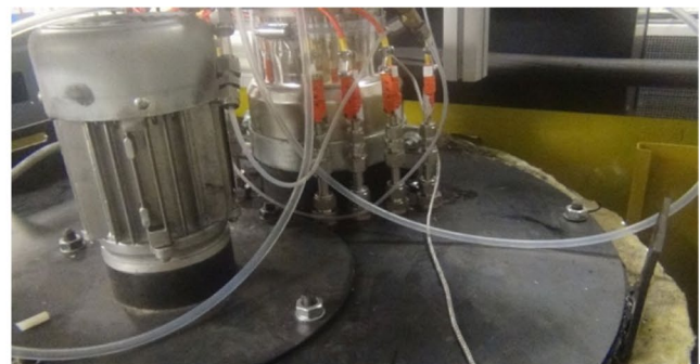
Fig. 2 Right: image of the thermocouples inserted from the top of the boiler in the second chamber. Center: front view of radial position and example of thermocouples heights (given in mm). Left: top view of radial position of the thermocouples
