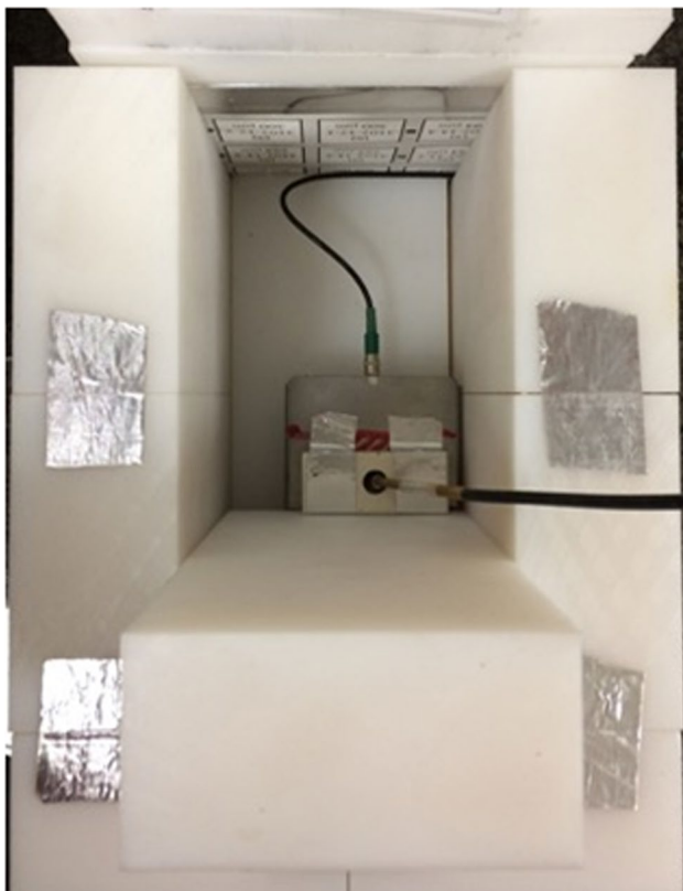
Fig. 2 Setup for neutron detection tests constituted by a moderator, made of polyethylene blocks, surrounding the detector box containing the ^{10}\text{B} neutron converter and the silicon diode (the moderator polyethylene top cover was removed to take the picture). The ^{252}\text{Cf} neutron source, handled by means of the black stick shown on the right, is inserted into the circular housing visible on top of the detector box
