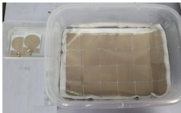
Fig. 9 CPW monopoles and AMC soaked into water for wetness measurement
