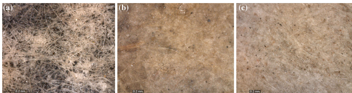
Fig. 2 USB microscope images ( \times 220 ) of: a original paper from the left portion of the cartoon; b French intervention paper; c original paper with patina from central portion of the cartoon ( staircase area)
