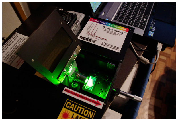
Fig. 1 A detail of the sampling stage of the Gem Raman instrument
