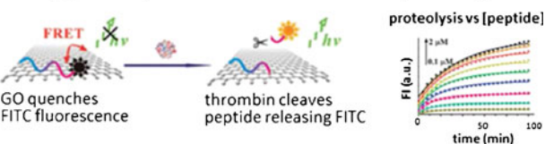
Fig. 2 Analytical devices based on biomolecule-graphene interfaces. a Functionalized graphene interface conductivity changes in response to bacterial binding. b A graphene oxide (GO)-peptide sensor monitors protease activity on the basis of an increase in fluorescence as fluorescein isothiocyanate (FITC) is released after peptide cleavage by thrombin. CFU colony-forming units, FI fluorescence, FRET fluorescence resonance energy transfer, IV intravenous. (Adapted with permission from [38, 41])
