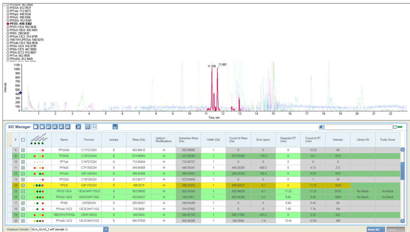
Fig. 3 Fish sample: PFOS was identified using the XIC Manager by accurate mass and isotopic profiling. The MS/MS spectrum also confirms the identity of the compound
